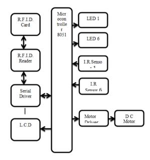
III. Working of Parking System using R.F.I.D
